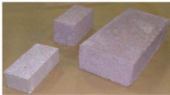
Picture 1. 2'x4'x8", 4'x8'x8", 4'x8'x16" CMUs, all dimensions are nominal. (Note: Regular CMU shown is not from 10' CMU, each surface shall be the same as the other CMUs.)
